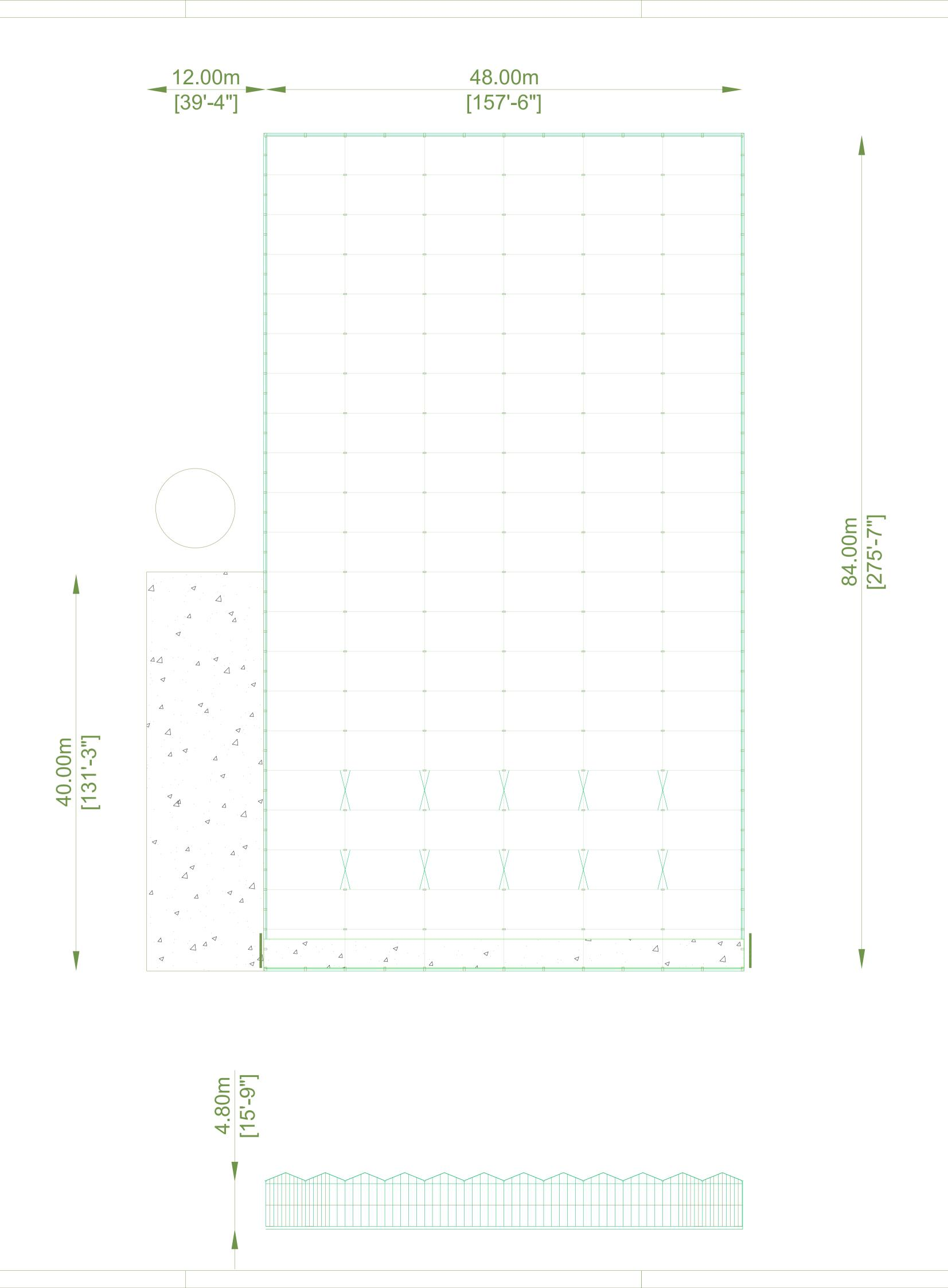
Expert 2.0 (21x [13 ft 1 in] = 275 ft 7 in) Length 275 ft 7 in 157 ft 6 in (6x [26 ft 3 in] = 157 ft 6 in) Width 43,400 sq ft 1.0 Acre Area 15 ft 9 in 7.31 psf Snow load<sup>1</sup>
