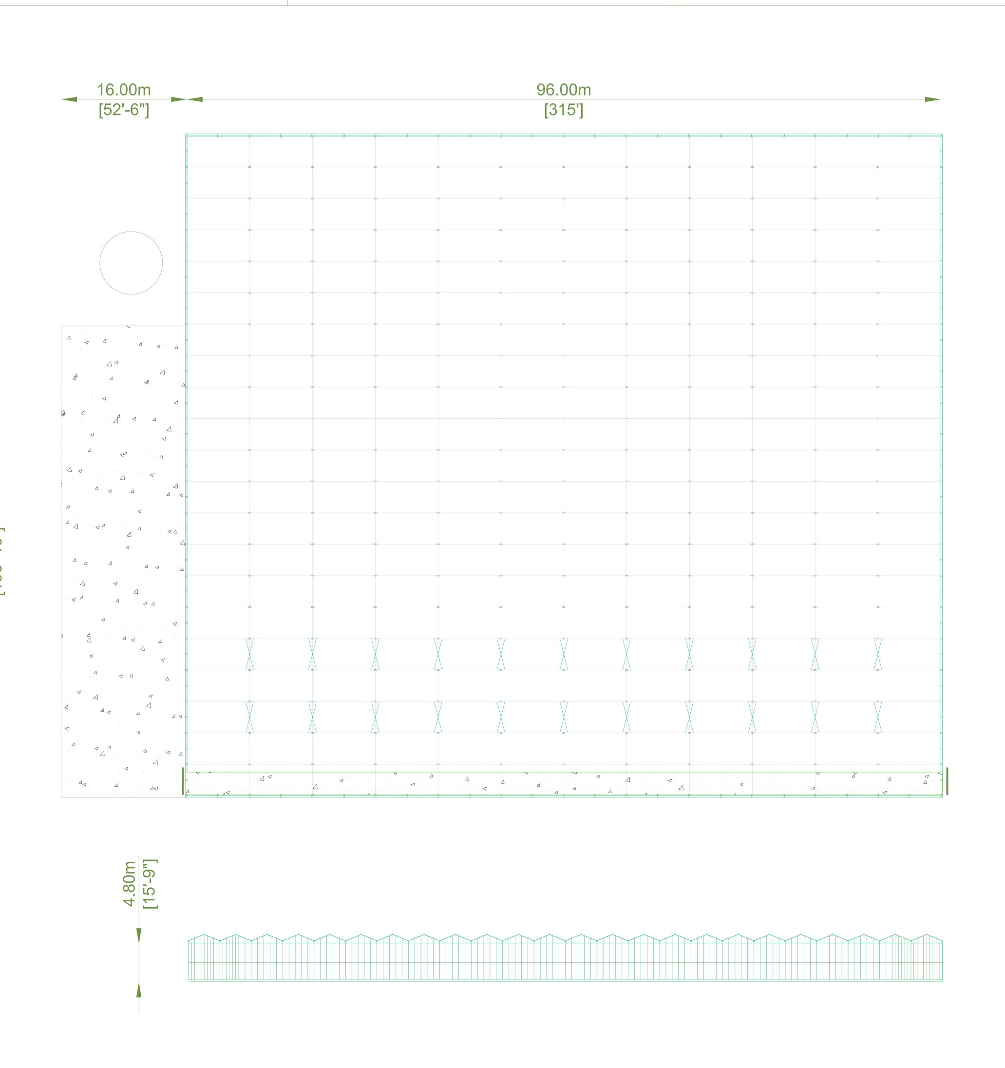
Expert 3.0 275 ft 7 in (21x [13 ft 1 in] = 275 ft 7 in) Length (12x [26 ft 3 in] = 315 ft) 315 ft Width 86,800 sq ft 2.0 Acre 15 ft 9 in 7.31 psf Snow load<sup>1</sup> 3.13 psf Crop load Installation loads 1.46 psf Windspeed<sup>2</sup> 105 mph
