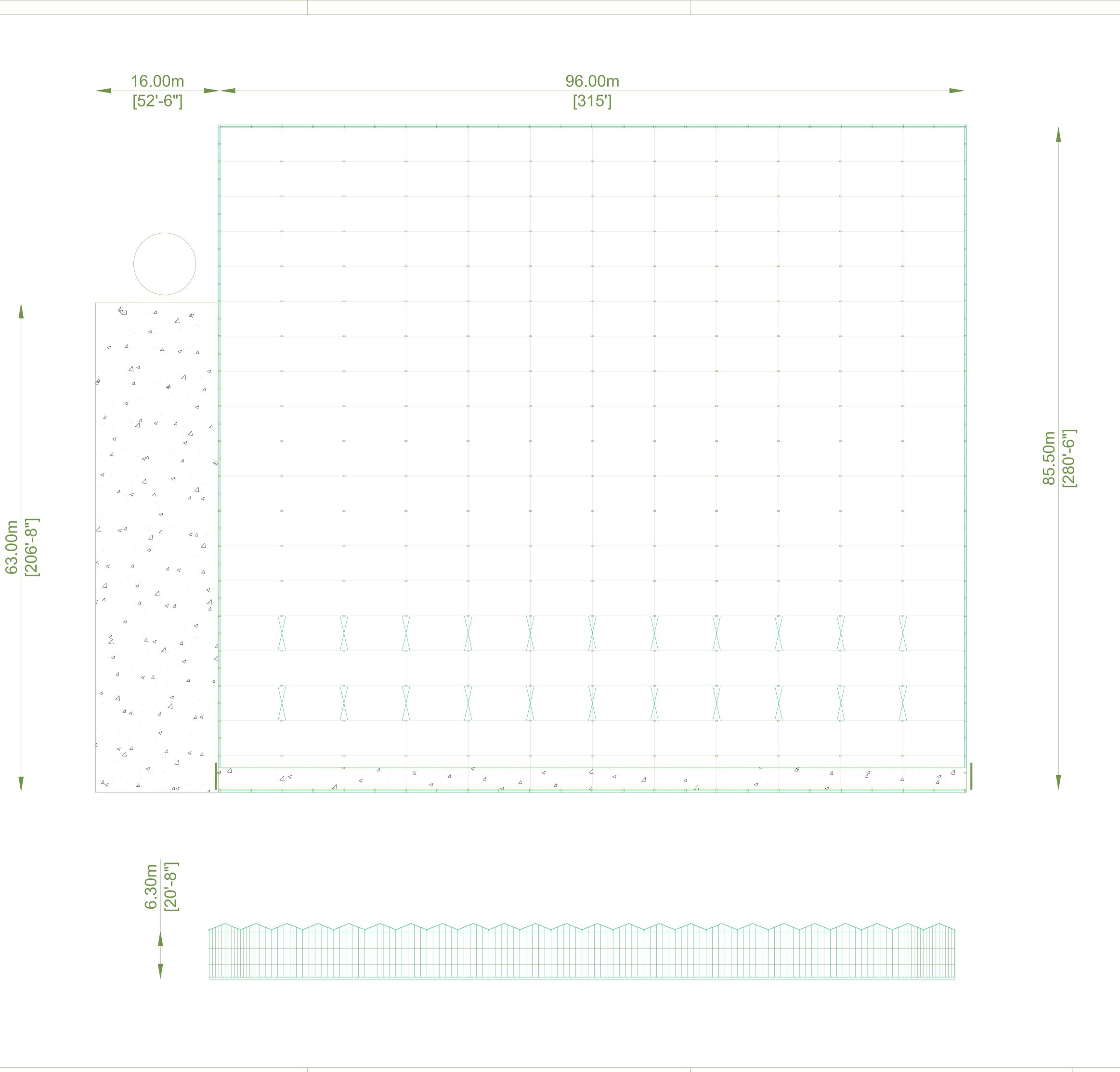
Plus 1.0 (19x [14 ft 9 in] = 280 ft 6 in) Length 280 ft 6 in (12x [26 ft 3 in] = 315 ft) Width 315 ft 88,350 sq ft 2.0 Acre 19 ft 8 in 7.31 psf Snow load<sup>1</sup> Crop load 4.18 psf Installation loads 1.46 psf Windspeed<sup>2</sup> 105 mph <sup>1</sup> In heavy snow areas a snow melt heating to be applied <sup>2</sup> Reduction factors apply
